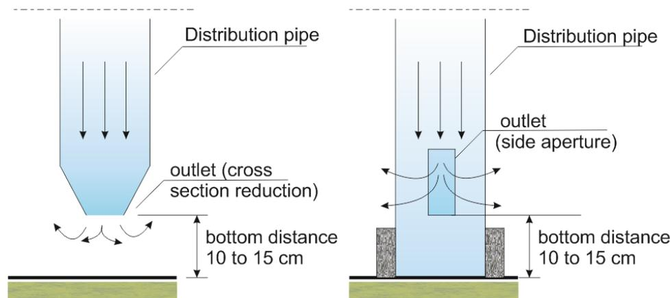
Figure 4.- Examples of distribution tube ends.
