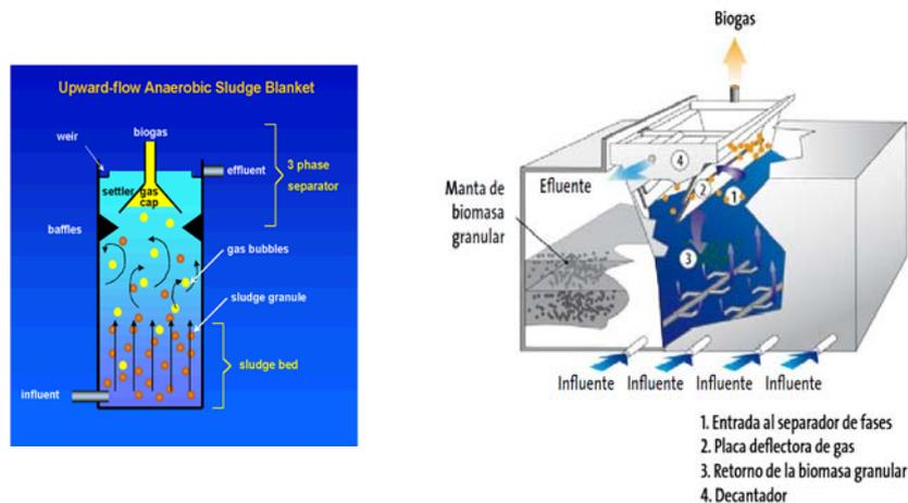
**Figure 1.- UASB reactors of the major anaerobic system manufacturers: (A) Paques, B.V. and (B) Biothane B.V.**
