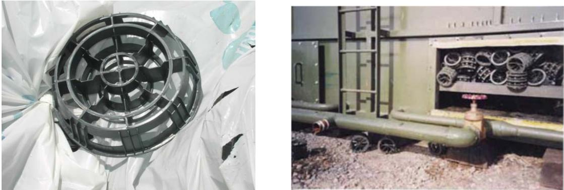
**Figure 4.- Right: Support media used in SAF processes used (average diameter: 12-15 cm). Left SAF unit filled with Pall-rings type bulk material (average diameter 9 cm).**
