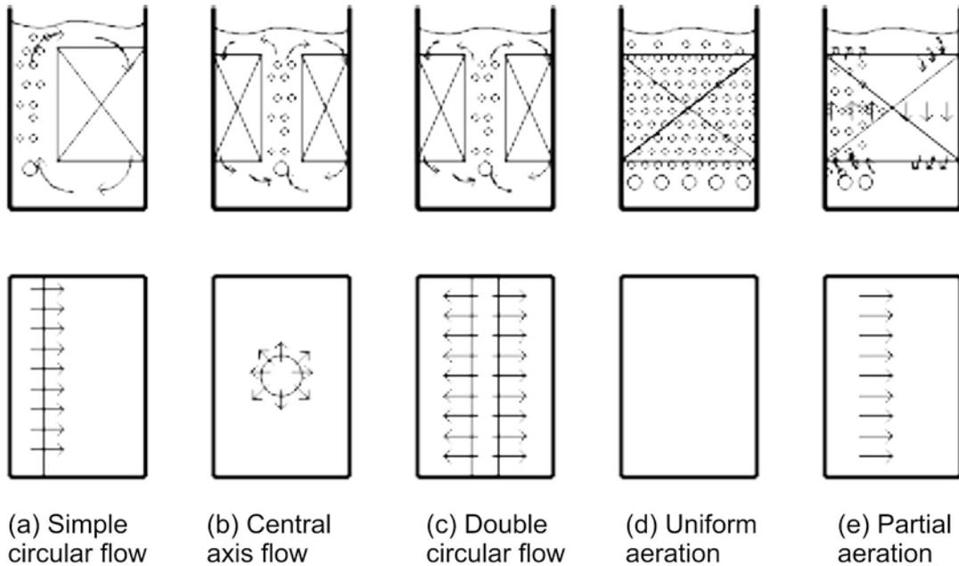
**Figure 7.- Types of aeration to submerged aerated filters(Reproduced from Iwai and Kitao, 1994)**
