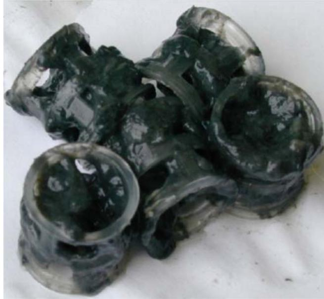
**Figure 10.- Biofilm grown on SAFTEX support media. This support is Pall-rings or similar type.**
