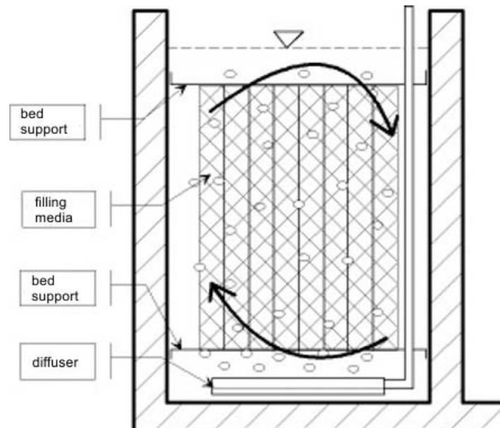
Figure 1. Scheme of a SAF process
