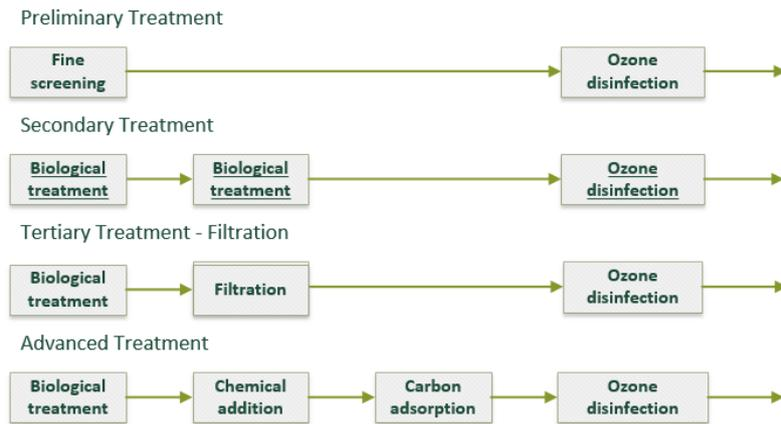
Figure 9 Ozone use schematic treatment examples (mod. from US EPA, 1986)
