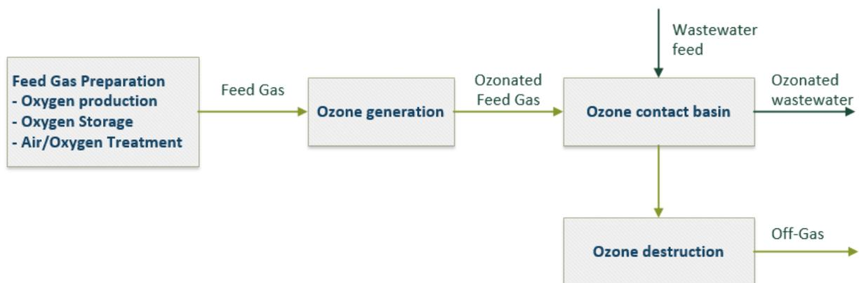
Figure 2. Simplified ozone process schematic diagram (mod. From US EPA, 1986)
