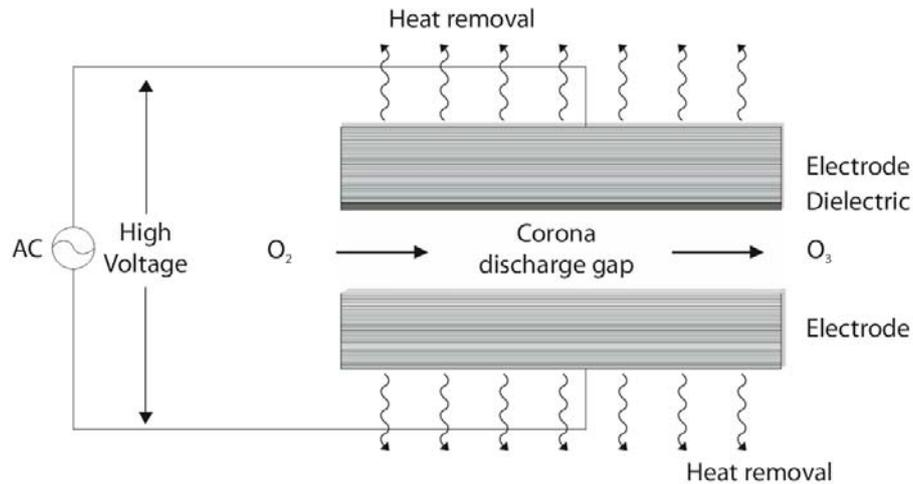
**Figure 5.- Principal elements of a corona discharge ozone generator (mod. from US EPA, 1986).**
