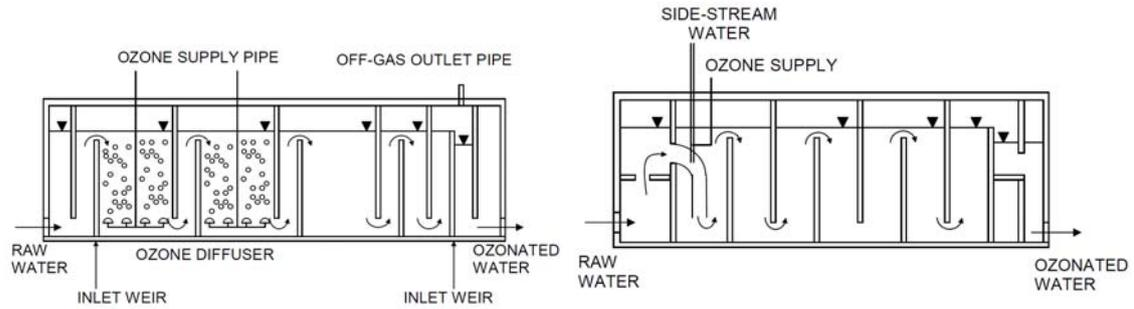
**Figure 6.- Sectional view of a fine bubble diffuser (left) and a sidestream water injector ozone contactor (Kim, 2007) .**
