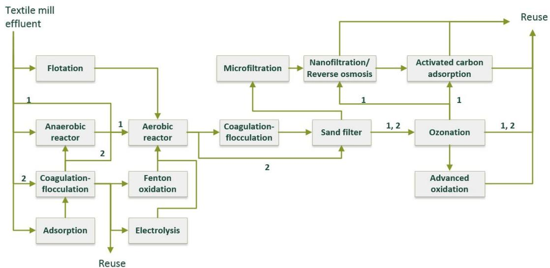
1: High Lura WWTP managed by CIDA Srl in the area of Como (Italy) treating 22,000 m<sup>3</sup>/d of a mixture consisting of 17% domestic WW, 32% rainwater, 51% textile finishing mill equalized effluent (cellulose, wool, silk and synthetic fibers). 2: Levi's Strauss WWTP, Wervik (Belgium).
