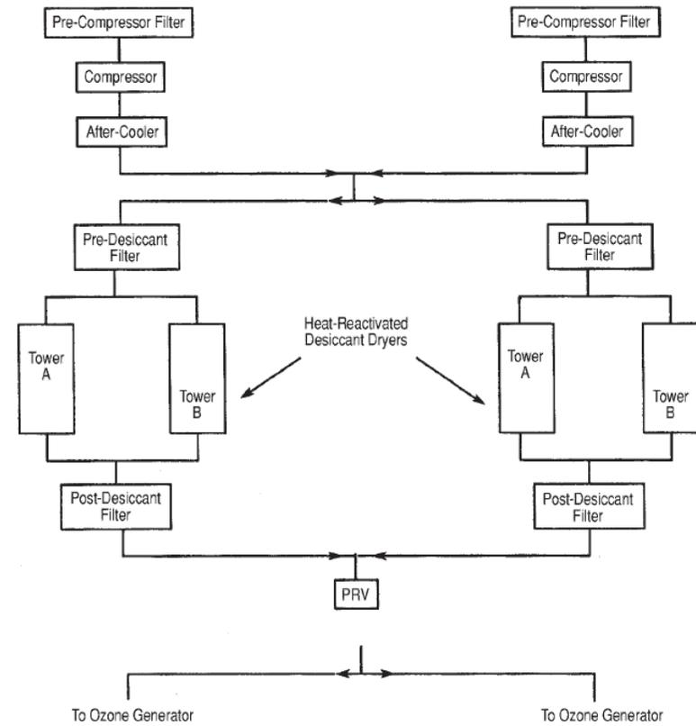
Figure 3.- Schematic diagrams for low (a) and high (b) pressure air feed gas treatment system (US EPA, 1986).
