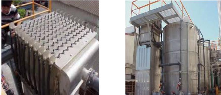
**Figure 5. Fered-Fenton reactor for the oxidation of non-biodegradable COD from a printboard factory in Taiwan (Ref.: ITRI, [www.itri.org.tw](http://www.itri.org.tw))**
