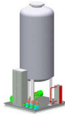
**Figure 10. Photograph and scheme of the treatment reactor for the catalytic Fenton oxidation treatment of segregated flow with high organic load in Schoeller Textiles AG (Switzerland), in operation since 1996 (Schömberger and Schäfer, 2003).**
