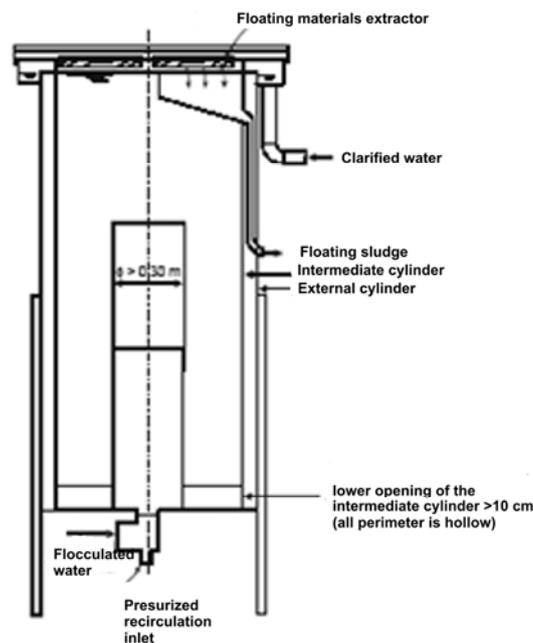
**Figure 8.- Circular flotation chamber.**
