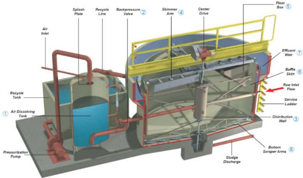
Figure 10.- Elements of a DAF system with a circular flotation chamber (ADVANCED ENERGY SOLUTIONS SAE LTDA.).
