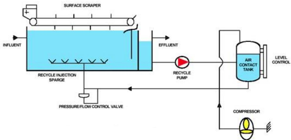
Figure 11.- Rectangular flotation tank scheme.
