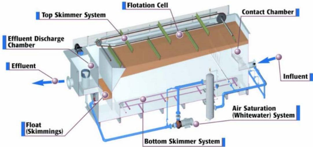
Figure 12.- Elements of a DAF system with rectangular flotation chamber (Ross, C., Valentine, GE et al. ; 2013).
