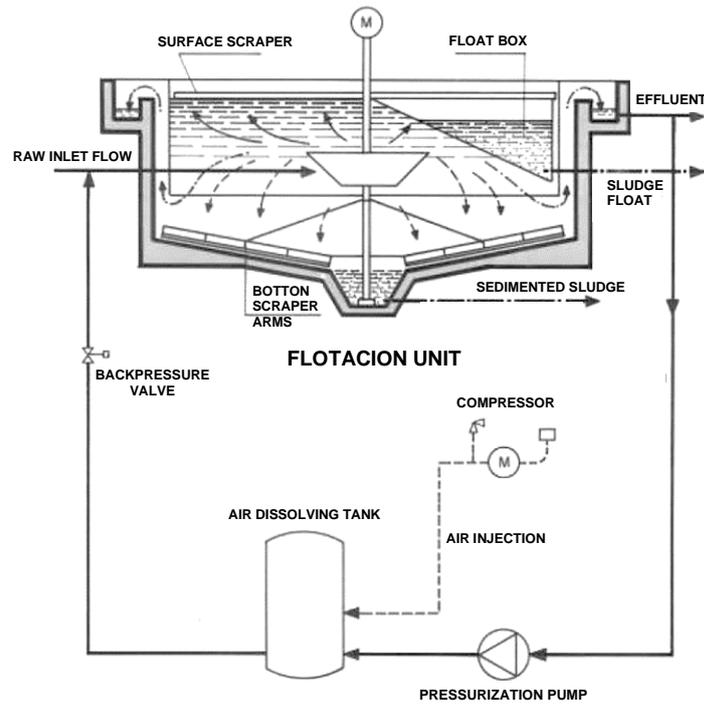
Figure 5.- Functional diagram of a circular DAF system.
