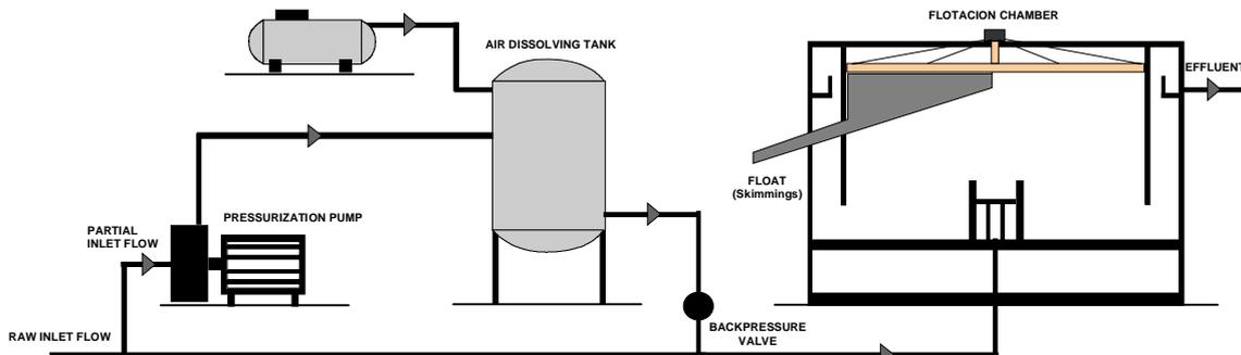
Figure 3.- DAF with partial inflow pressurization (CEPIS, 1992).
