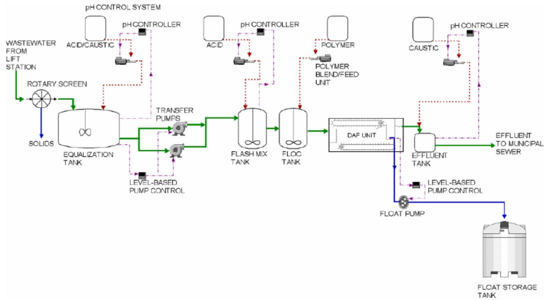
Figure 13.- Integration of a DAF system in a WWTP pretreatment (Ross, C., Valentine, GE et al. ; 2013).
