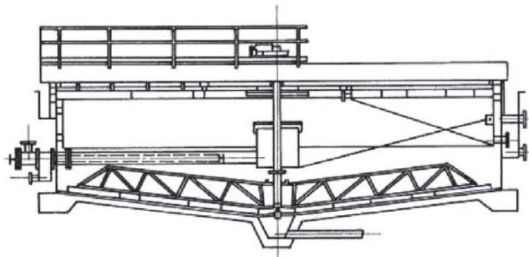
**Figure 9.- Circular flotation tank floor scheme**
