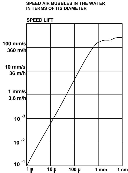
Figure 1.- Vertical speed of air bubbles as a function of diameter.
