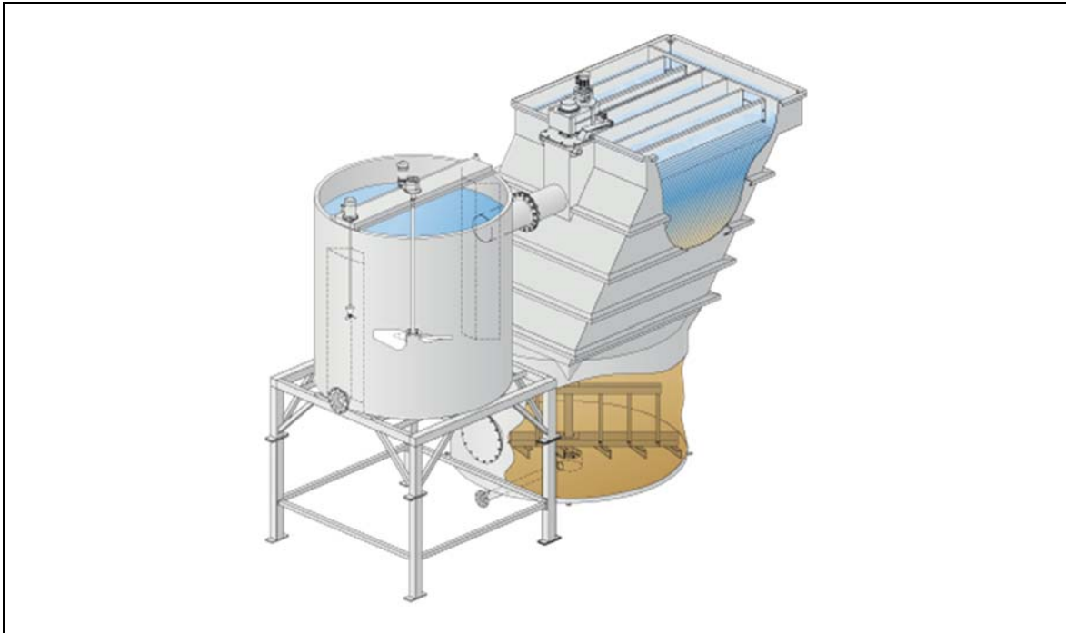
Figure 11 Flocculation chamber and lamella separator.
