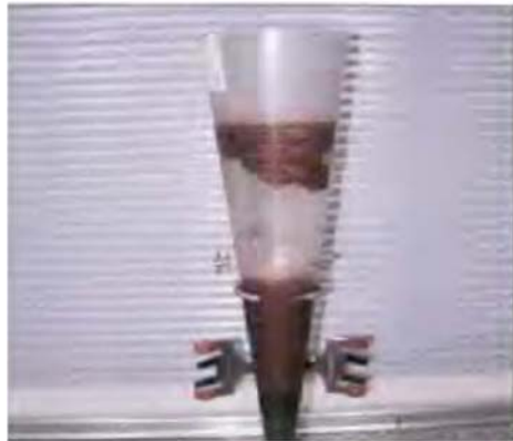
Figure 6.- Floated sludge after several hours of testing V30.
