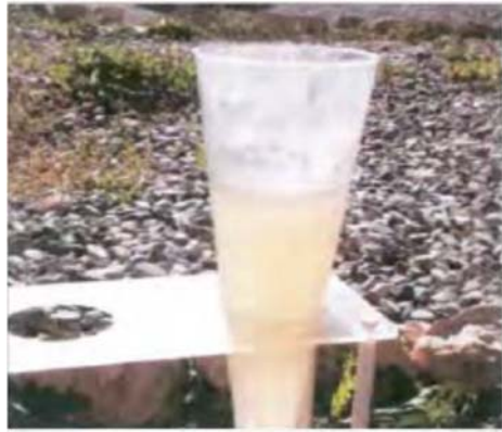
Figure 4.- Yellowish secondary clarified effluent.
