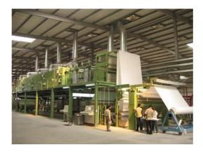
It is possible to create modular mega-machines which combine bleaching, mercerising, washing, drying, dyeing, fixing, washing and drying into a single machine several hundred meters long.
