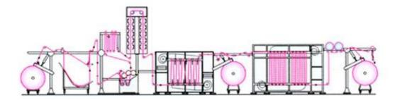
Continuous dyeing ranges tend to have several sections that use very large amounts of energy per hour – if fabric is being processed the energy per metre is low but lots of energy is wasted when the machine is not actually processing fabric.
