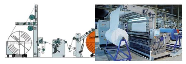
The fabric is dipped in a trough containing dye and alkali (typically sodium hydroxide and/or sodium silicate), it is mangled and then wound on a roll without drying it.
