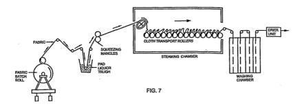
In order to get good dye fixation in the limited time the fabric has in either a steamer or thermofix unit it is often necessary to add humectants (chemicals that attract moisture), such as urea, to the dye liquor in addition to the alkali used for dye fixation. Urea in effluent is a major problem because it is difficult to remediate (it requires specific denitrification techniques) and if discharged to the environment it acts as unwanted fertiliser and can cause damaging algal blooms.
